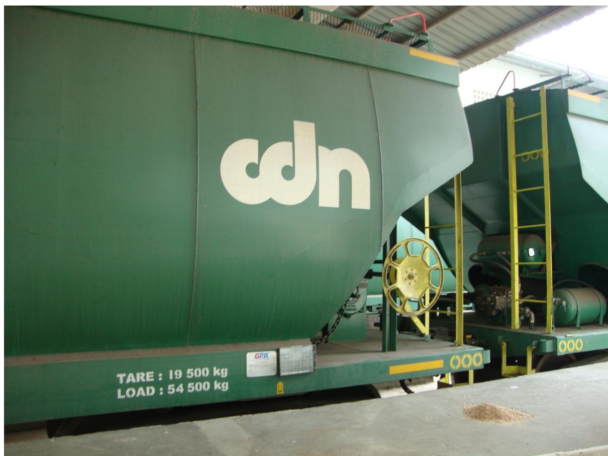
FIGURE 36: NEW CDN GRAIN WAGON 54.5T LOAD, BUT LIMITED TO 40T BECAUSE OF THE 15T AXLE
